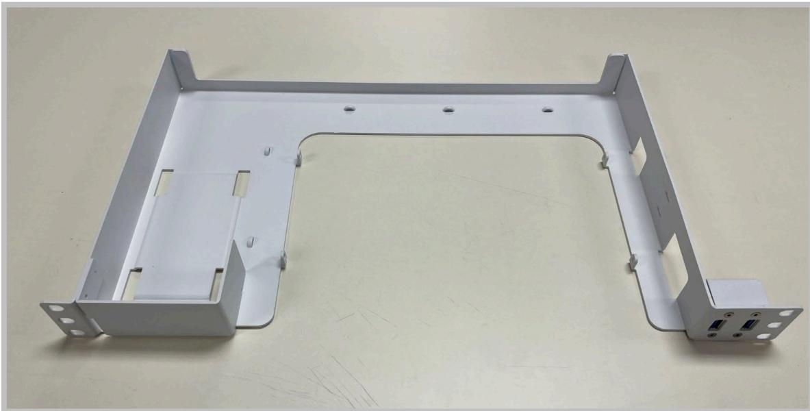
2. Align the mounting holes in the X1600 Socket with the holes located in the tabs on the rackmount bracket.
