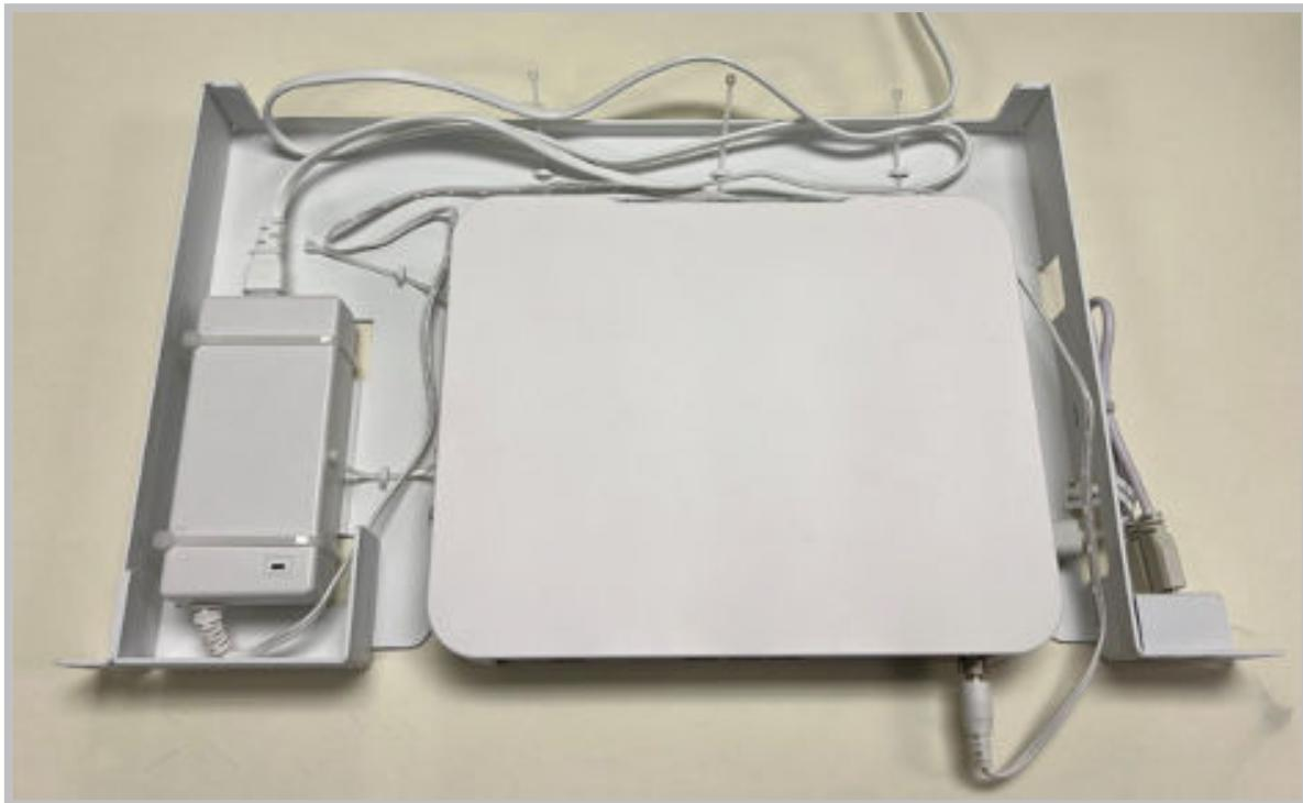
10. Secure the PSU cables with the cable ties. If necessary, bundle any excess cable slack and secure with the remaining 99mm cable tie. Snip off the excess.
