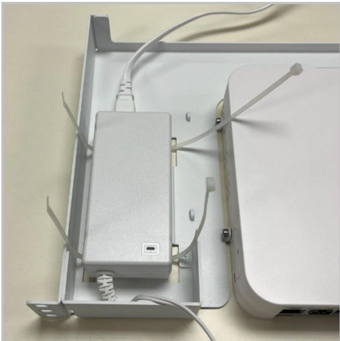
8. Secure the PSU to the rackmount bracket with the cable ties and snip of the excess. Screw the power cable into the X1600 Socket.
