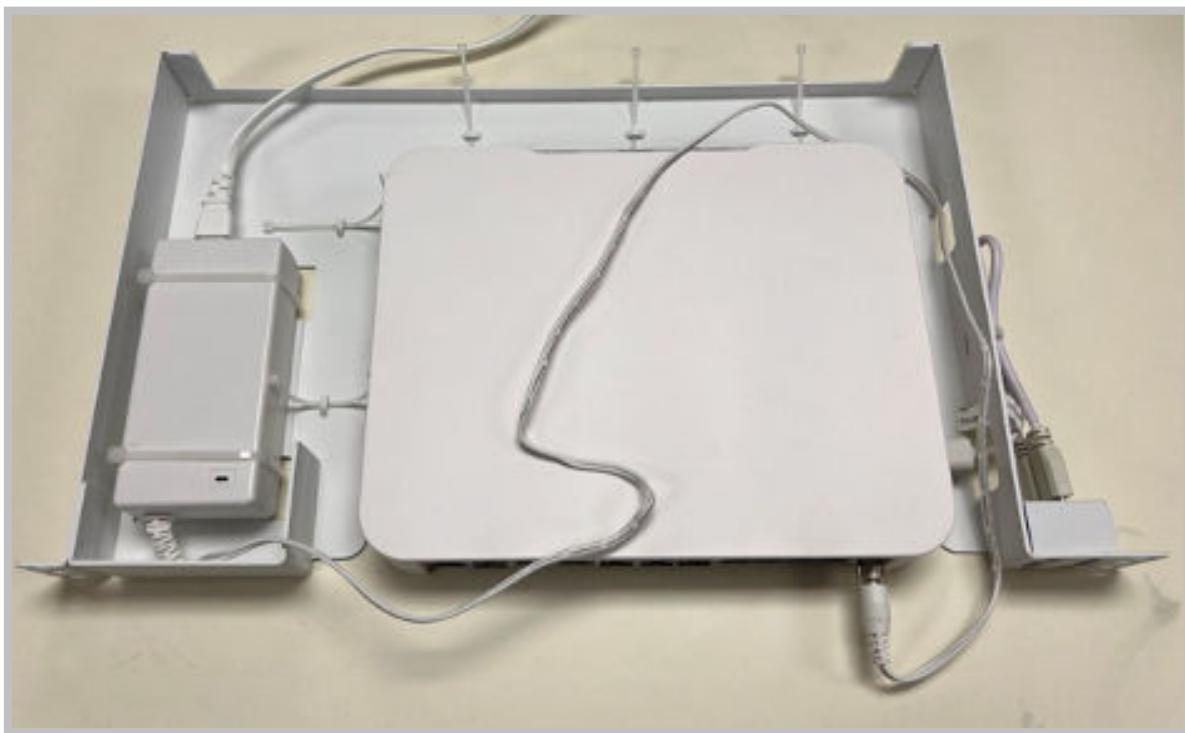
Bundle the PSU cables and route them around the rackmount bracket as shown.
