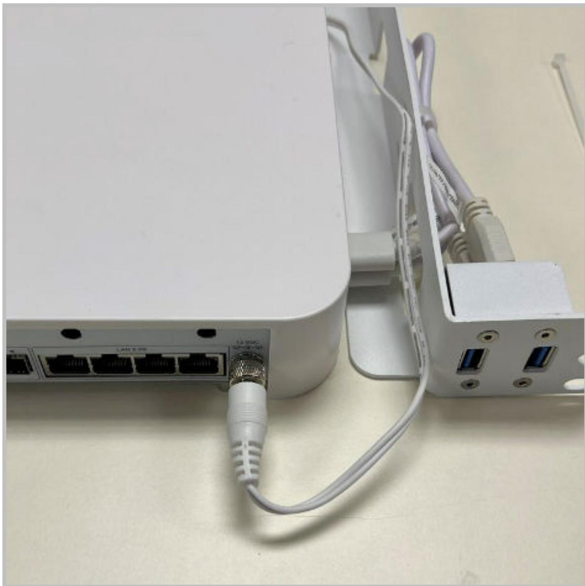
9. Route five 99mm cable ties through the cable tie mounts on the rackmount bracket where shown.
