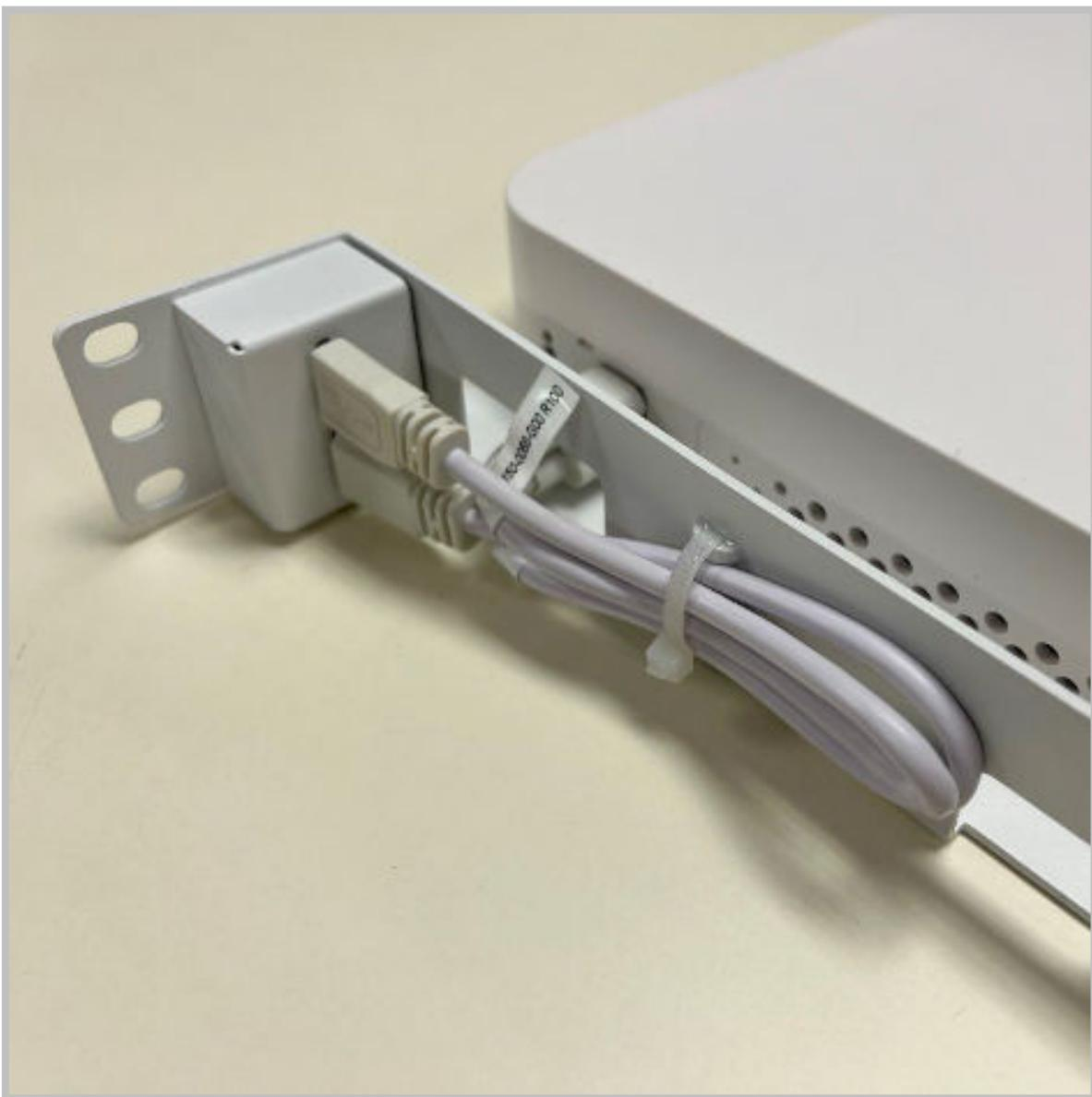
7. Route two 300mm cable ties underneath the PSU standoff on the rackmount bracket. Place the PSU on the standoff with the cables oriented as shown.
