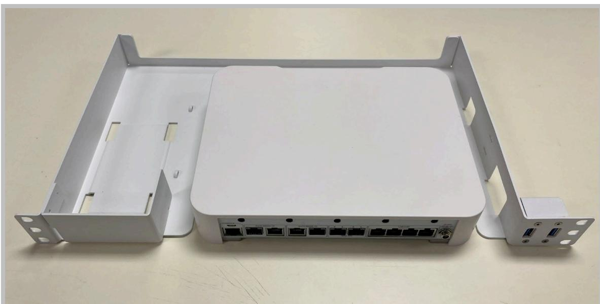
3. Insert a screw into one of the mounting holes and snug. Do not overtighten.
