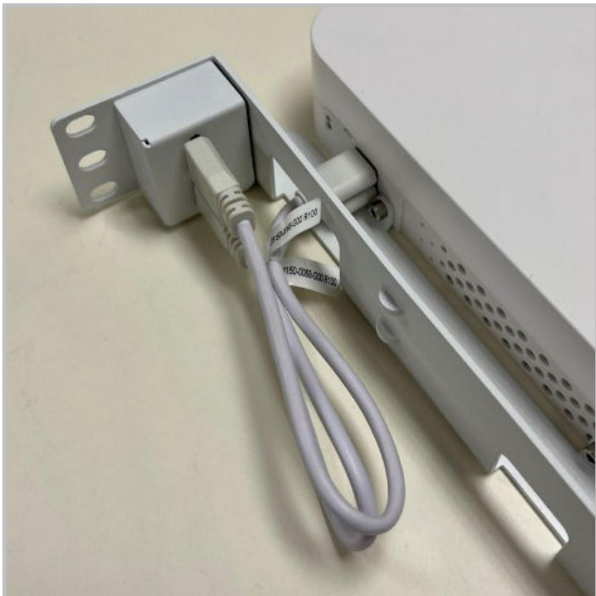
6. Secure the cables in place with a 300mm cable tie passed through the cable tie mounts on the rackmount bracket and snip off the excess.
