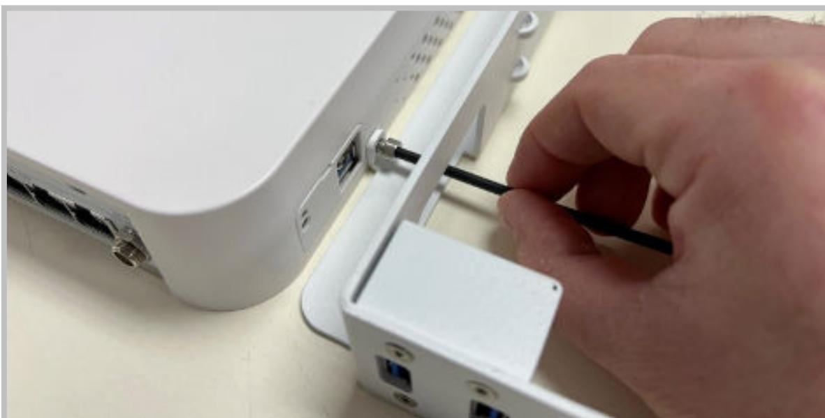
4. Insert the remaining screws into the mounting holes and snug. Do not overtighten.
