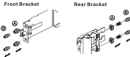
4) Fix the outer rail/bracket assembly to the frame.
