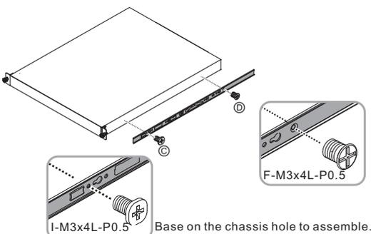
3) Check hole type on rack post. Choose suitable pin of bracket to install if needed.
