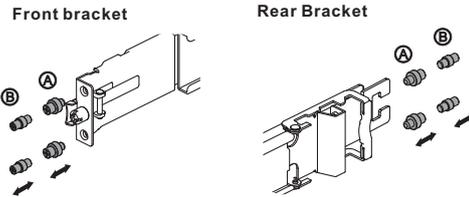
4) Fix the outer rail/bracket assembly to the frame.
