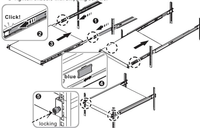
Remove the chassis from rack.
