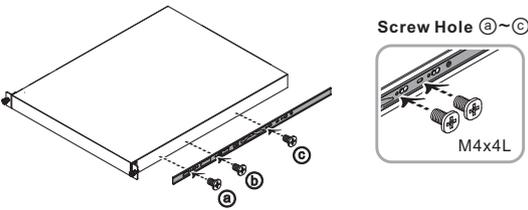
3) Check hole type on rack post. Choose suitable pin of bracket to install if needed.
