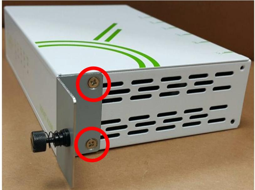
2. Use two screws (D) to secure the second Cato Socket X1500 side bracket (C) to the left side of the Cato Socket X1500.
