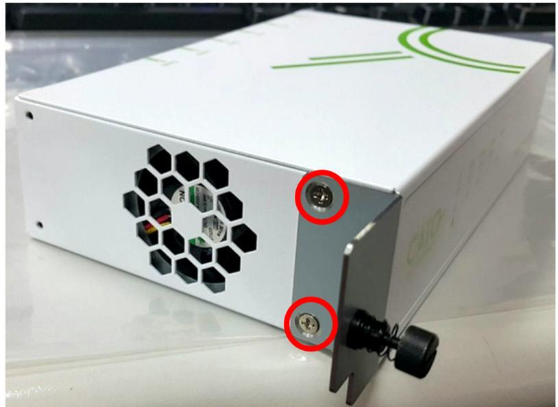
3. Place the Cato Socket X1500 with the side brackets at the front of the shelf and secure to the shelf using the side bracket thumb screws on both sides.
