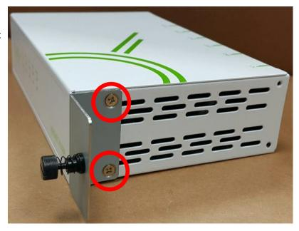
2. Use two screws (D) to secure the second Cato Socket X1500 side bracket (C) to the left side of the Cato Socket X1500.
