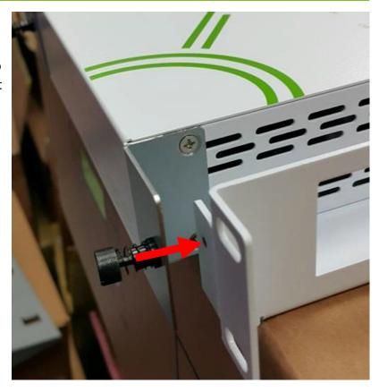
To mount another Cato Socket X1500 and its power supply in the shelf, repeat the steps in Section 3.1 - Mounting the Cato Socket X1500 Power Adapter and Section 3.2 - Mounting the Cato Socket X1500
