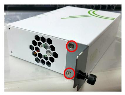
3. Place the Cato Socket X1500 with the side brackets at the front of the shelf and secure to the shelf using the side bracket thumb screws on both sides.
